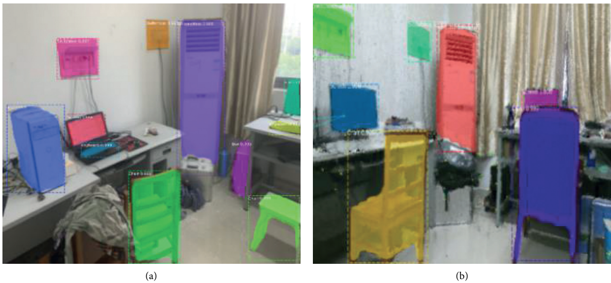
FIGURE 7: Effect image of target detection and recognition (a) and semantic map of dense point cloud (b).
