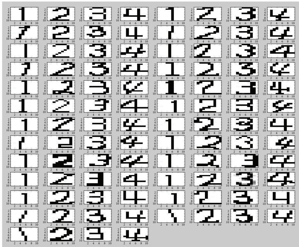
FIGURE 7: The picture of 100 different patterns of alphanumeric letters 1, 2, 3, and 4 used in the optical character recognition experiment.
