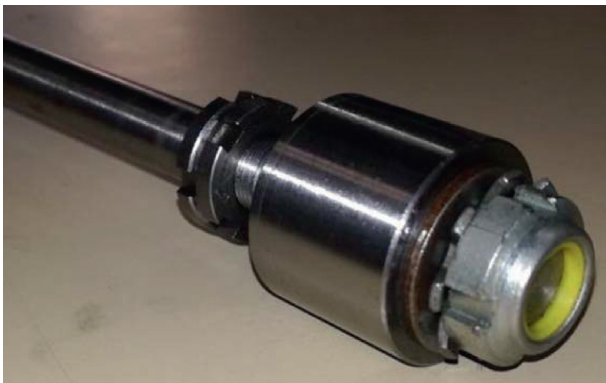
FIGURE 3: Prototype of the custom shaft with interchangeable journals.
