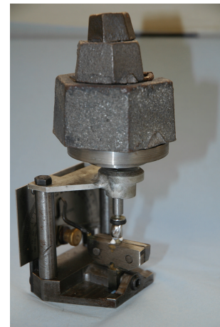
FIGURE 6: Cementation of a crown under static load.
