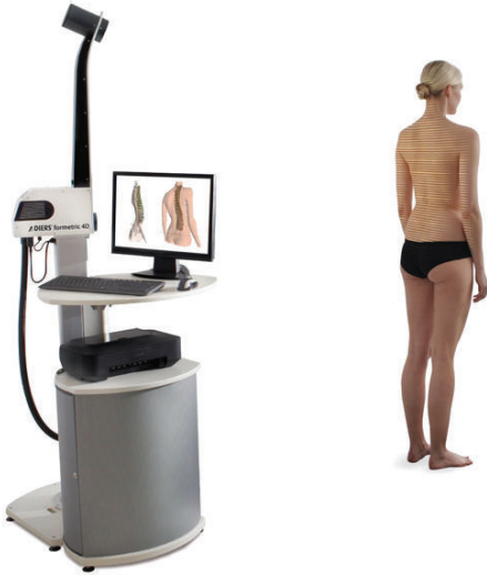
FIGURE 3: Formetric 4D device with raster line projection.
