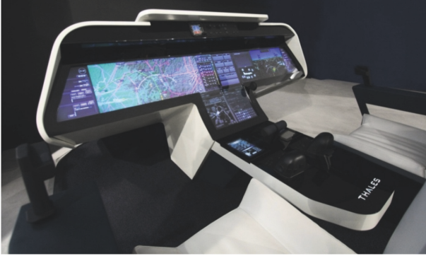
FIGURE 1: A picture of a prototype of future aircraft cockpit as envisioned by the ODICIS project (Copyright Thales Aerospace).
